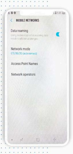
Make sure that **Data Roaming** is **ON** then tap on **Access Point Names** and tap on **ADD**.
