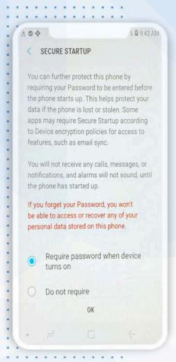
In Android settings tap on Security then on Secure Startup. Make sure that Require password when device turns on is selected then choose OK and confirm by entering the device's password.
